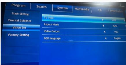
Recommendation: For using RCA the recommended "TV Type" 480i.
